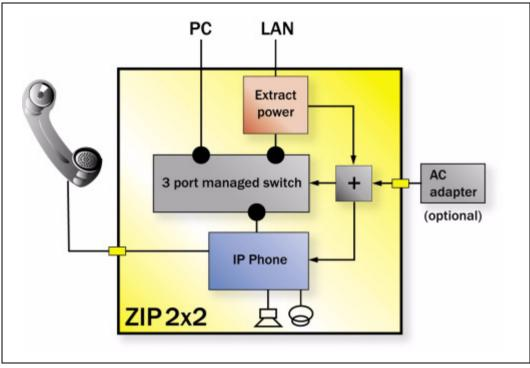
Figure 1-3 Internal Representation of the ZIP2x2 Managed Switch
