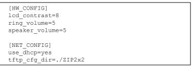
Figure C-2 Configuration File Example
