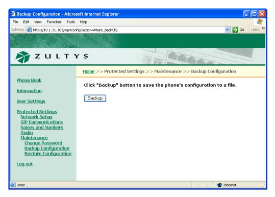
Figure E-23 Maintenance – Backup Configuration panel
