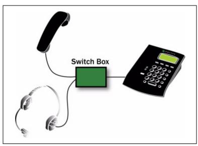
Figure 3-5 Connecting a Headset to the Phone Using an External Switch Box
