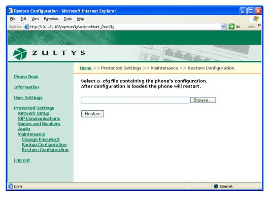
Figure E-24 Maintenance – Restore Configuration panel
