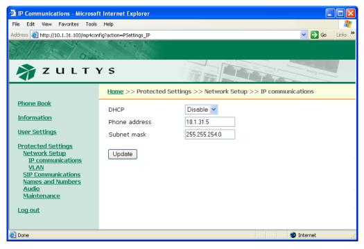
Figure E-17 Protected Settings – IP Communications panel
